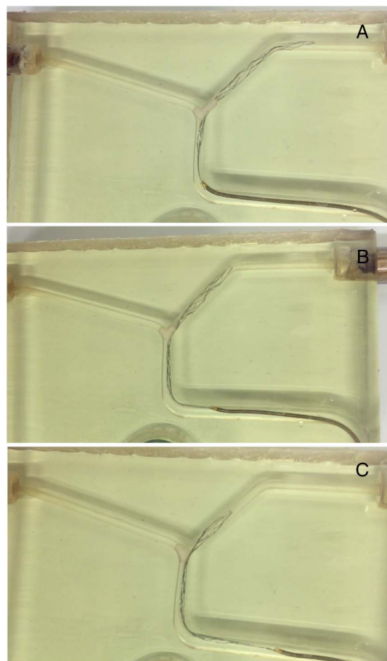
Figure 4 Interaction between Solitaire 4–20 and a large white clot: interaction of the proximal, middle, and distal thirds of the device (A–C).
